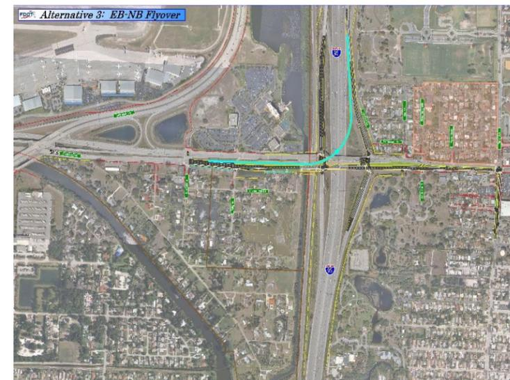
**Alternative 3: EB SR 80 to NB I-95 Flyover:** Single-lane third level ramp from EB SR 80 to NB I-95. Requires R/W from the south side of SR 80, west of I-95.
